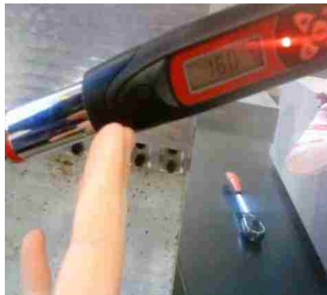
Figure 9: Digital torque wrench for tightening bolts
