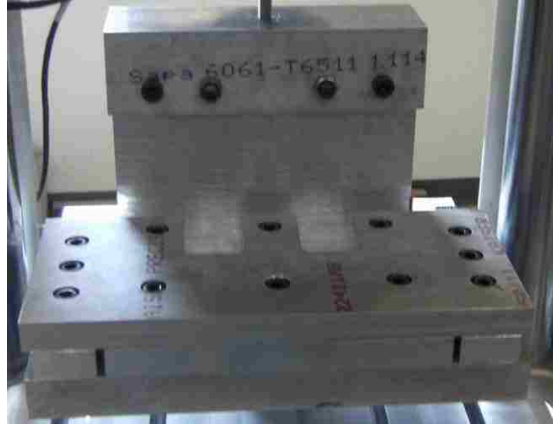
Figure 7: Test Article for measuring local shear slip
